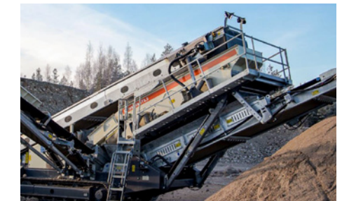
Platforms and emergency wires for improved safety.
