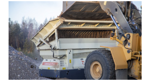
Tipping/vibrating grid for separating oversize material.
