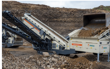
Large feed box allows closed circuit process.
