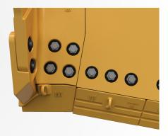
When half arrows are at half-life, replace the corner segment edges with new half-life corner segment edges.
