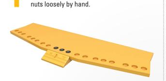
Install the center half arrow to base edge using nuts, washers, and bolts. Tighten the
